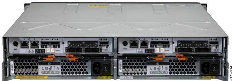
Figure 21. TS7720 Cache Drawer 3956-XS9 (rear view)
