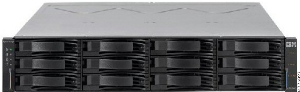
Figure 20. TS7720 Cache Drawer 3956-XS9 (front view)
